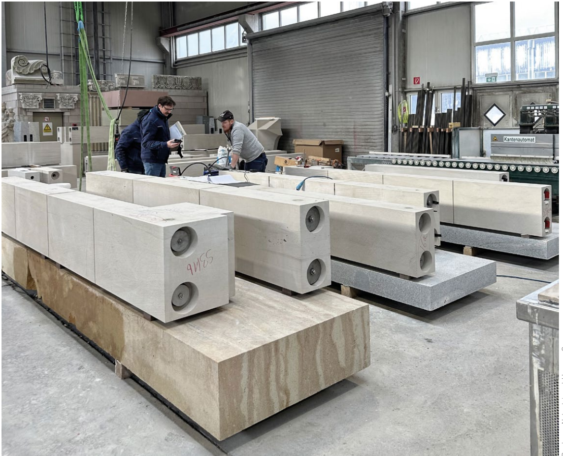
Prestressed lintels with spans of up to 5 m at the workshop of Bamberger Natursteinwerk, Germany.
